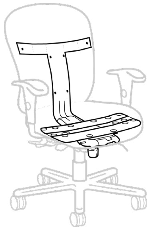
Steel Support Structure
