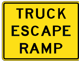
W7-4C TRUCK ESCAPE RAMP (SPECIFY ARROW)
