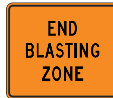
W22-3 END BLASTING ZONE
