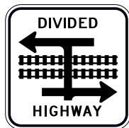
R15-7A DIVIDED HIGHWAY T-INTERSECTION OVER TRACKS 24"
