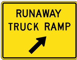
W7-4B TRUCK ESCAPE RAMP W/ARROW
