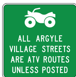
D1-10A ATV ROUTE NOTIFICATION ( SPECIFY NAME) 24" • 36"
