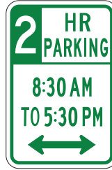
R7-108D LIMITED PARKING (GREEN CORNER) (SPECIFY DURATION/ TIMES)(SPECIFY ARROW) 12" x 18"
