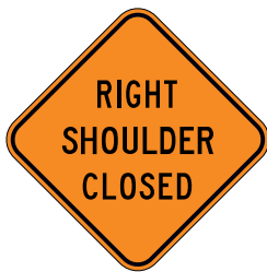
W21-5A SHOULDER CLOSED (SPECIFY DIRECTION)
