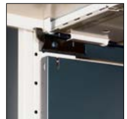
Receding Door Mechanism uses nylon glides to prevent metal-to-metal contact, allowing smooth motion.
