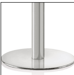
Disk Pedestal Base - features a 4" column composed of .04" thick steel with a welded reinforcement.
