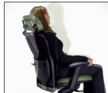
Breathe features a synchronized knee-tilt mechanism with a 2:1 ratio (back-to-seat). Tilt-lock lever can be positioned to 5 different lock positions or remain unlocked for free-float function.
