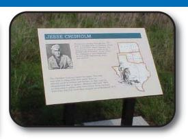
**Pedestal** interpretive mounts provide a flat plate for sign mounting (no frame), with a 48" tall aluminum 4"  $\times$  4" post, and 48" steel tubing posts (3"  $\times$  3") with mounting plates to be installed in ground to support the aluminum posts and sign. Customer chooses a viewing angle of 45, 60, or 90 degrees.
